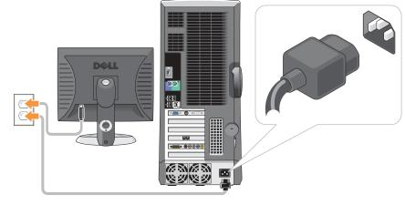
Connect the computer and monitor to electrical outlets.
