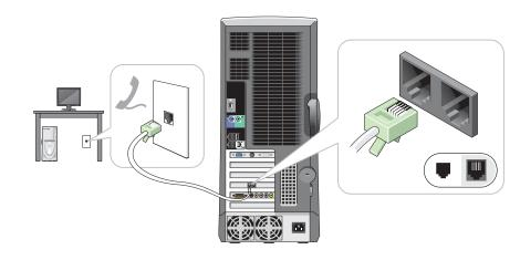
If you have a modem, connect a telephone cable to either of the modem connectors. Do not connect the telephone cable to the network connector.
