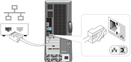
If you have a network device, connect a network cable (not included) to the network connector.
